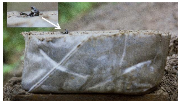
Figures 15 and 16. The minimal front surface of the hunting tip is the reason for the full penetration of a 30 cm sandbag - notice the arrow tip!
